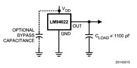
FIGURE 2. LM94022 No Decoupling Required for Capacitive Loads Less than 1100 pF.
