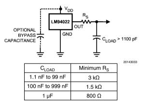
FIGURE 3. LM94022 with series resistor for capacitive Loading greater than 1100 pF.
